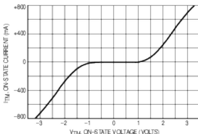
Figure 2. On-State Characteristics
