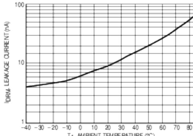
Figure 6. Leakage Current, I<sub>DRM</sub> versus Temperature
