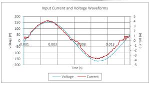
Input AC Current Waveform (ITHD = 9.54%, 50% Load)
